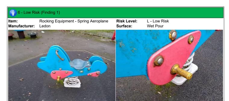
**Finding:** The end of footrests have a cross section of less than 15cm2 and fail to meet the requirements of BS EN 1176 Part 6
