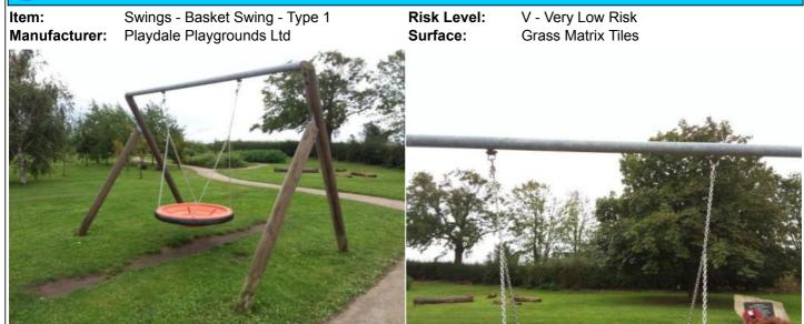
**Finding:** Swings of this design should have a secondary after the regularly safety mechanism fitted to prevent collapse of the seat in the regularly event of a joint failure to comply with BS EN 1176 Part 2, however this swing was installed prior to the standards being updated in 2018 and the manufacturer has confirmed that the joint was independently cycle tested by BSi
