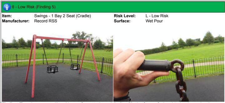
Finding: There is some notable evidence of wear to the anti Action: Monitor for any further deterioration and replace wrap bars when 40% worn
